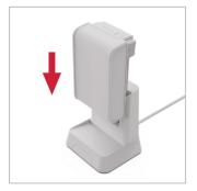
Plug in the charger. Attach the battery pack to the charger by aligning the ribs on the battery pack to the grooves in the charger.
