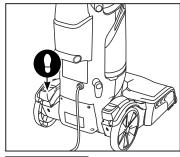
2 Grab the Dirty Water Tank handle and pull up to release. Remove Tank from carpet cleaner base at an angle.
